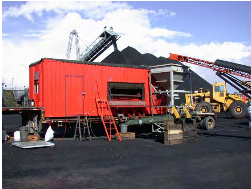
Figure 3. On-site test set-up using the 5 tph FGX pilot-scale air table.
