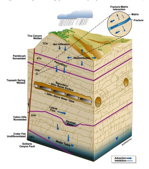
Figure 3. Conceptual drawing of mountain-scale flow processes (CRWMS, 2000a)
