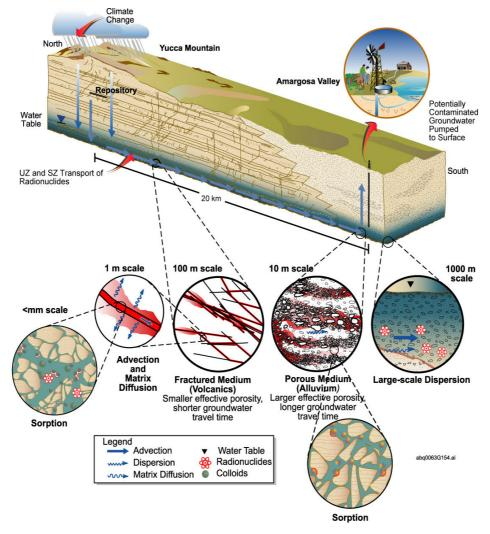
Figure 4. Conceptualisation of features and processes important to saturated zone transport (CRWMS, 2000a).
